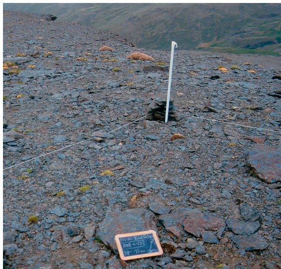
Fig. 4.7 A corner point of a summit area section . The 10m-point ( p10m-W ) on Pico del Tosal Cartujo (Sierra Nevada/Spain, 3150m a.s.l.) is marked with a signal rod for photo documentation .
